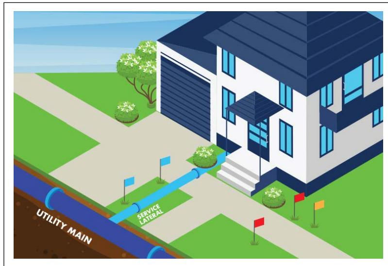
**A new Illinois law requires any existing service lateral that is completely replaced or any newly installed lateral to be made locatable by electromagnetic or other equally effective means for marking the location of the service lateral.**
